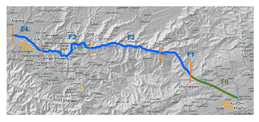
In sum, construction of up to 51.6 km road is planned on Rikoti Pass, including 96 bridges and 53 tunnels. Construction of Rikoti Pass section is divided into four sections: Chumateleti-Khevi section (section I) 11.7 km, Khevi-Ubisa section (section II) 12.2 km, Ubisa-Shorapani section (section III) 13 km and Shorapani-Argveta section (section IV) 14.7 km.
